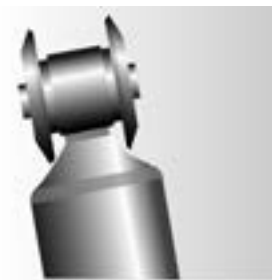
Improper installation Example: washer (if equipped) installed backwards
