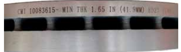
Offset rotor with one rotor plate thicker than the other. The part number is stamped onto edge 10016195 – 2007 to 2018 – ABS ring 10 Bolt 10083615 – 2018 – ABS ring 5 Bolt 10084701 – 2019 onwards – ABS ring with Circlip
