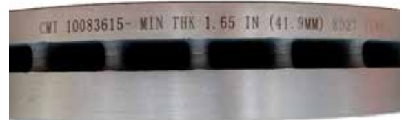
Offset rotor with one rotor plate thicker than the other.
