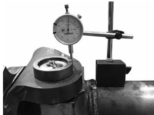
Figure 28: Checking steering knuckle vertical end play
