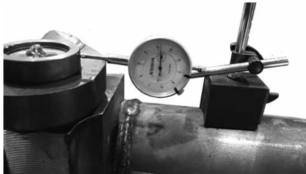
Figure 15: Checking upper kingpin bushing
