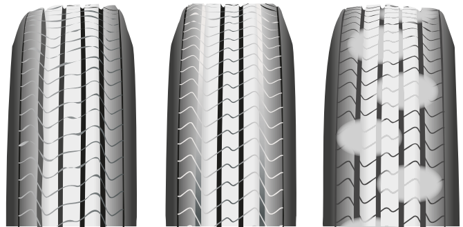
Figure 219: Feathered, Edge Wear, Cupped Wear Patterns
