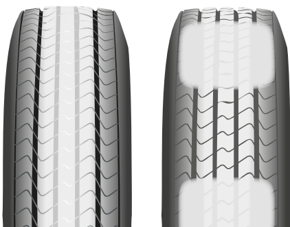
Figure 218: Centre Wear & Flat Spot Tyre Wear Patterns
