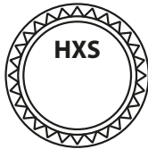
Figure 67: HXS is Stamped into the End of the S-Cam
