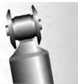
Improper installation Example: washer (if equipped installed backwards)
