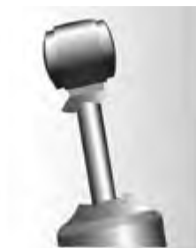
Damaged dust cover and / or shock body
