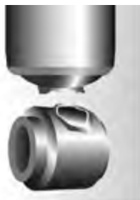
Damaged upper or lower mount
