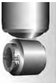
Damaged upper or lower bushing
