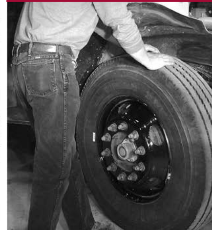
MOVE BOTTOM OF TIRE IN AND OUT
