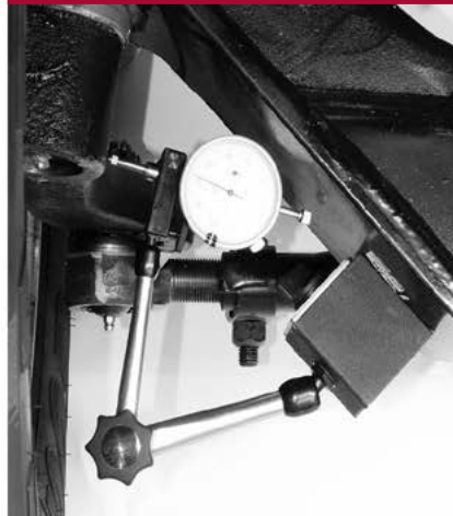
CHECK LOWER KINGPIN BUSHING
