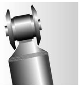
Improper intallation Example: washer (if equipped installed backwards
