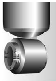
Damaged upper or lower bushing
