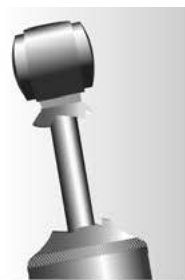
Damaged dust cover and / or shock body
