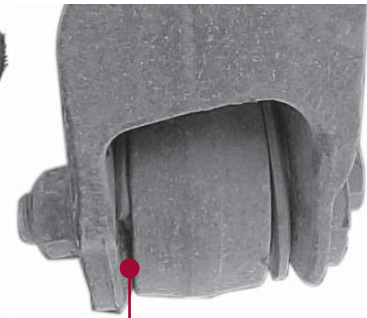
Missing Rubber Flange
