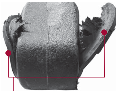
Disconnected Rubber Flange
