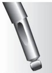
Bent or dented shock
