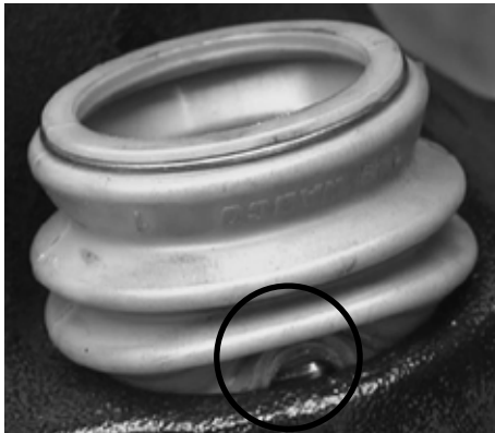
Figure 25: Improperly seated guide pin boot
