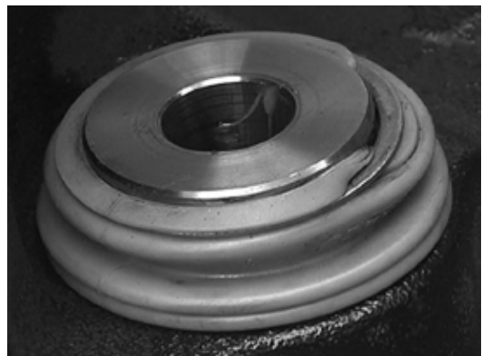
Figure 62: Improper seating of guide pin boot on guide pin
