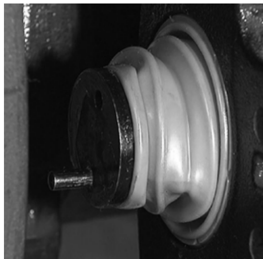
Figure 28: Wrinkled adjuster piston boot
