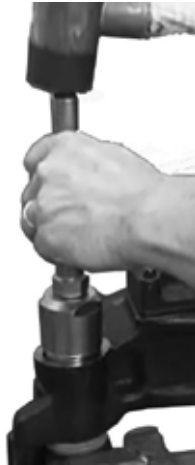
Figure 70: Using tool to install guide pin cap
