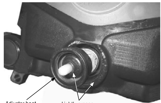
Figure 83: Installing adjuster boot
