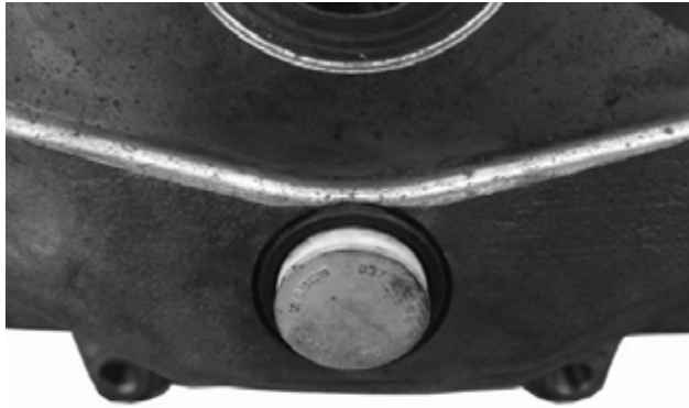
Figure 88: Adjuster plug properly inserted
