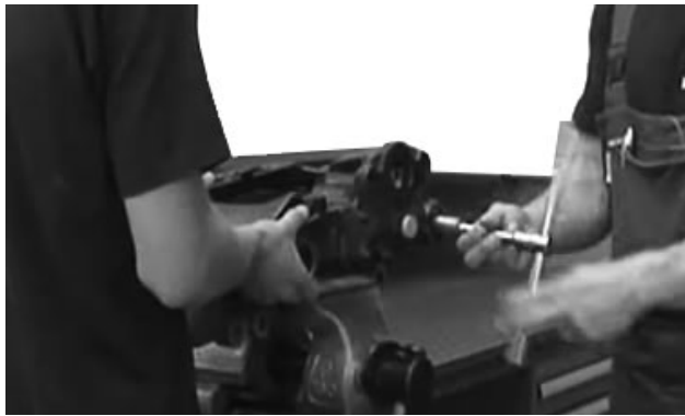
Figure 50: Supporting caliper while removing screws
