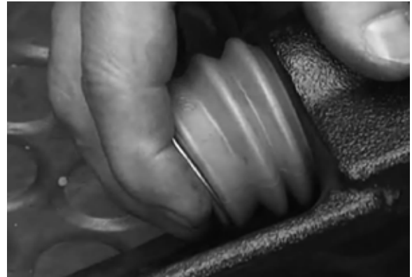
Figure 60: Seating of guide pin boot on guide pin
