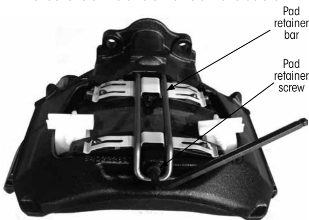
Figure 16: Removing pad retainer screw
