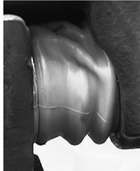
Figure 26: Twisted guide pin boot
