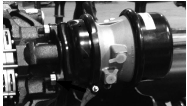
Figure 46: Installing brake chamber
