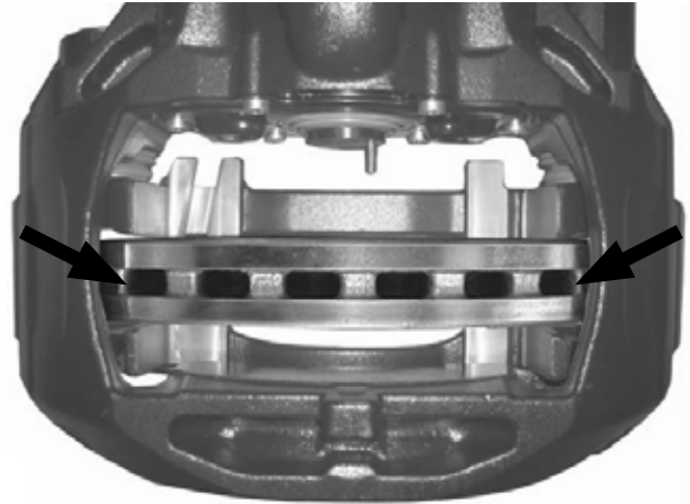
Figure 40: Positioning caliper over brake rotor
