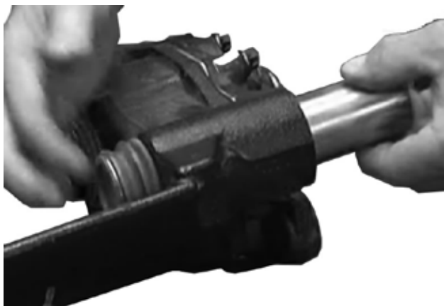
Figure 59: Inserting guide pin
