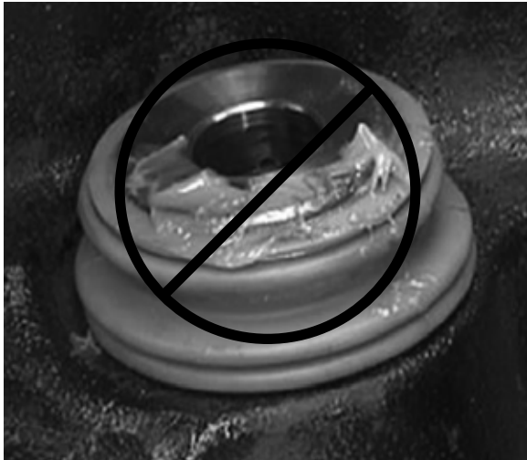
Figure 63: Excessive grease on guide pin and boot
