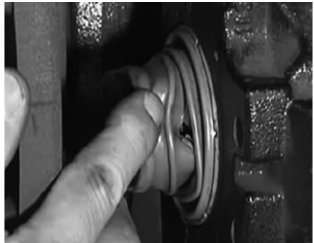
Figure 27: Adjuster piston boot damage
