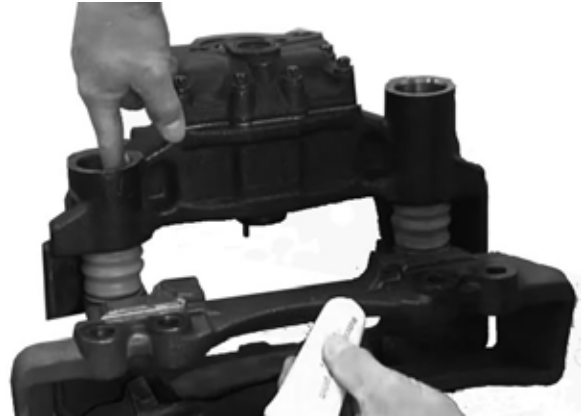
Figure 68: Greasing bore of guide pin cap
