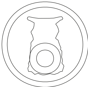
Figure 12: Bush in Need of Replacement (Inner Metal Separation)
