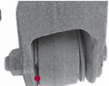
Missing Rubber Flange
