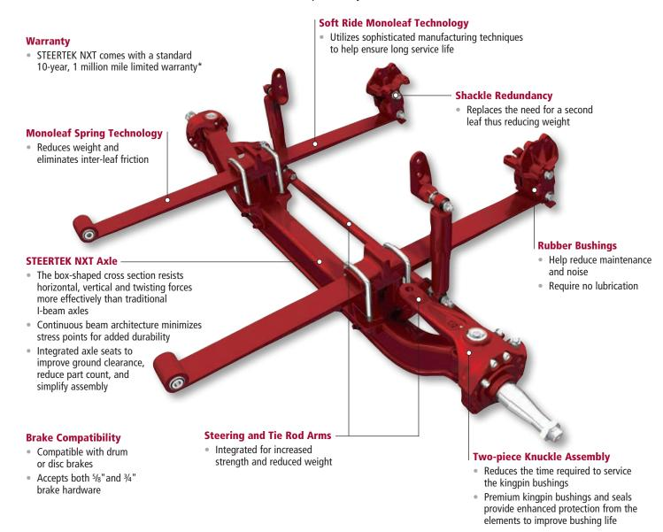
All applications must be pre-approved by both Hendrickson and vehicle manufacturer. SOFTEK is integral to and available exclusively with the STEERTEK NXT axle. Contact Hendrickson or vehicle manufacturer for availability.
