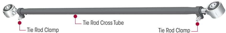
2. Rotate the cross tube to achieve the recommended  $\frac{1}{16}$ " to  $\frac{1}{8}$ " toe-in specification.
