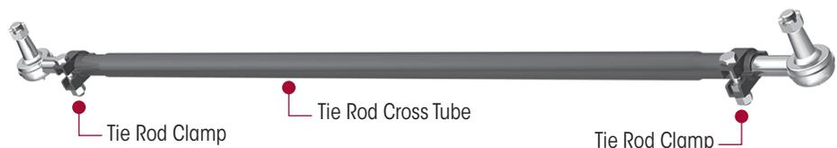
2. Rotate the cross tube to achieve the recommended  $\frac{1}{16}$ " to  $\frac{1}{8}$ " toe-in specification.
