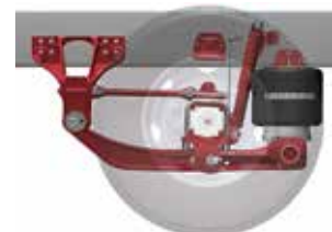
Protected shock and air spring (shown with 11R 22.5 tire)
