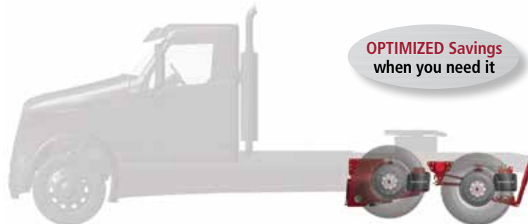
Axle lifted for 4×2 configuration — The OPTIMAAX system senses lighter load conditions and lifts the non-drive axle
