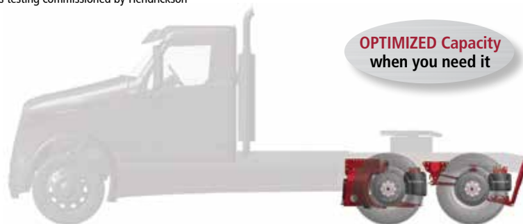
Axle lowered for 6×2 configuration — The OPTIMAAX system senses higher load conditions and lowers the non-drive axle
