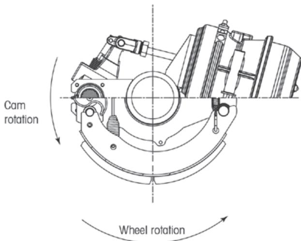
Figure 1: Cam and wheels must rotate in the same direction
